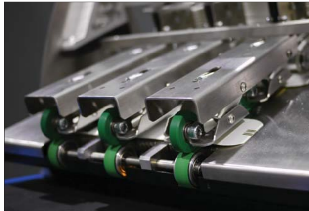
Self adjusting exit rollers.
